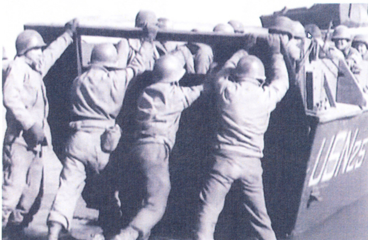
Infantry load up in LCVP for the crossing. Apparently the ramp winch is defective as it is manually lifted. Joakim Steinweden
