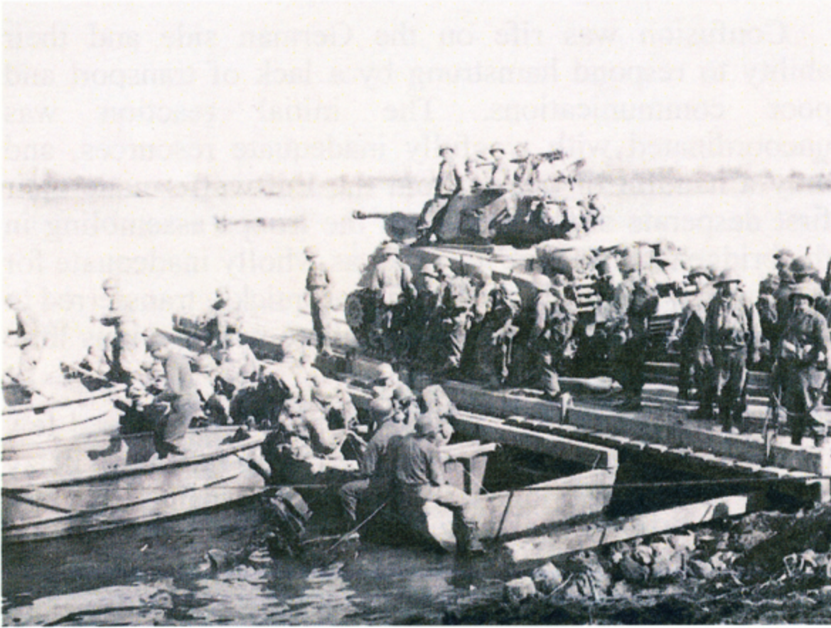
An M-4A3E8 Sherman tank is loaded onto a ferry for the river crossing. Signal Corps
